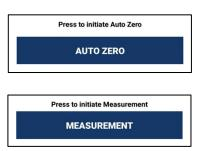
Prior to any sample measurement at the start of a new method, an auto zero measurement of either water or the buffer of the samples is required to give the Photopette a reference of what zero should be.
