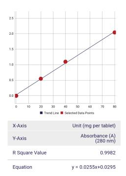
**Figure 2:** Calibration curve from "Method Maker" showing perfect linearity and large measurement range.
